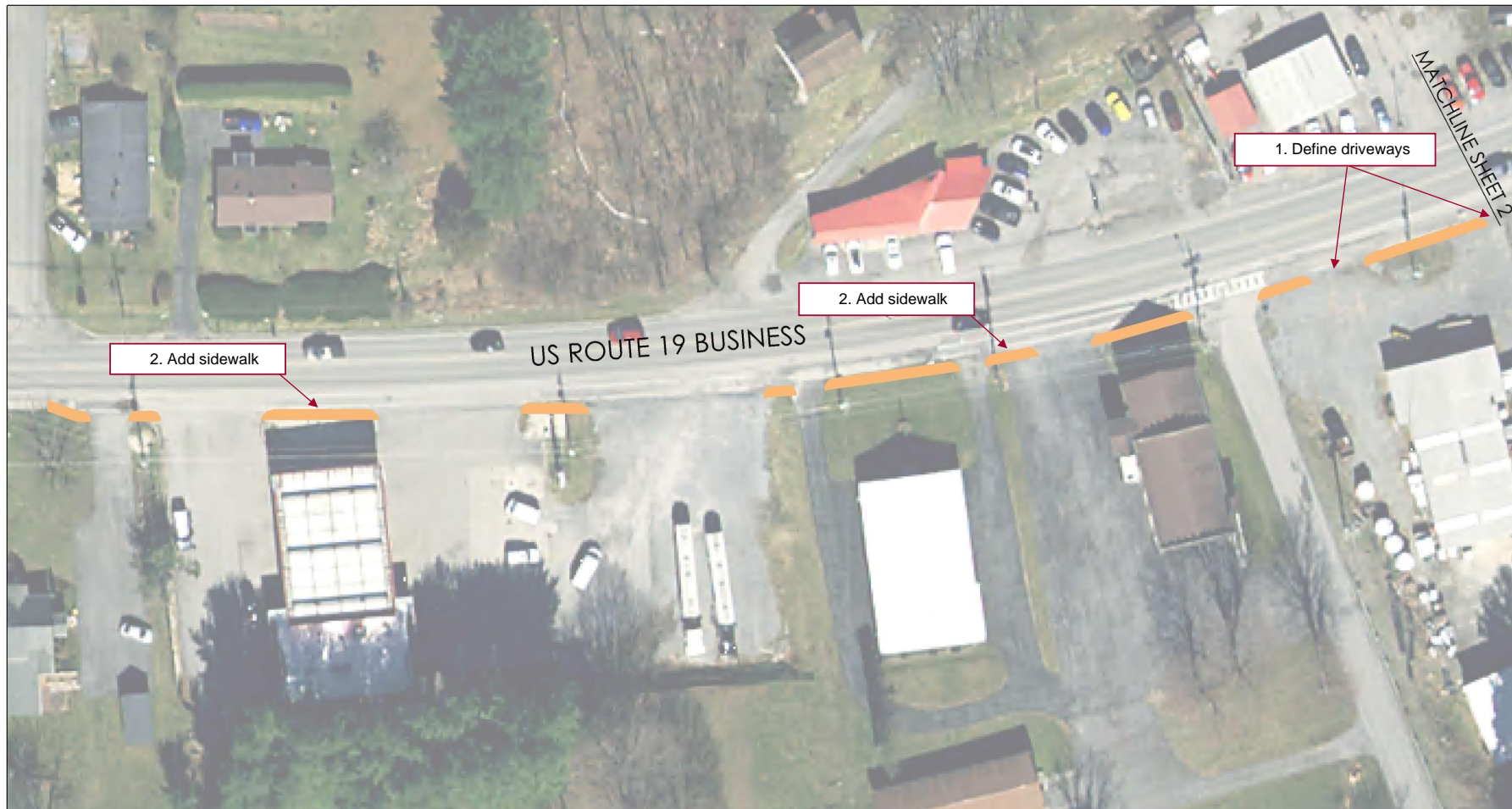
Figure 6. Long-Term Intersection Improvements Sheet 1
